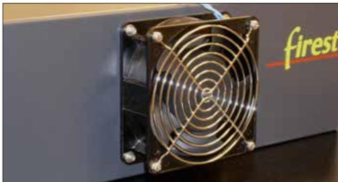
Maintaining the recommended operating temperatures for sealed CO<sub>2</sub> lasers is critical. The use of secondary cooling mechanisms like fans or flowing water systems are commonly added to assist cooling.
