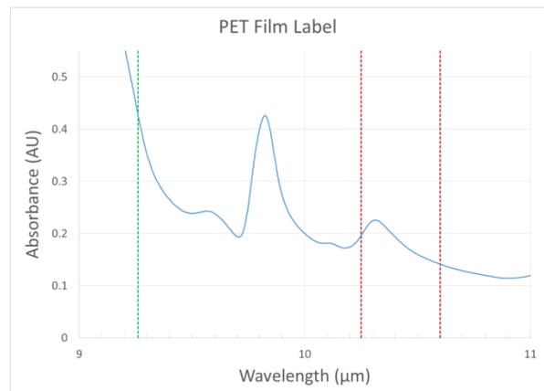
Figure 5: A measured FT-IR absorbance curve of a PET label. From left to right, the 3 vertical lines indicate the 9.3  $\mu\text{m}$ , 10.2  $\mu\text{m}$ , and 10.6  $\mu\text{m}$  wavelengths. Green color code indicates the best absorption.
