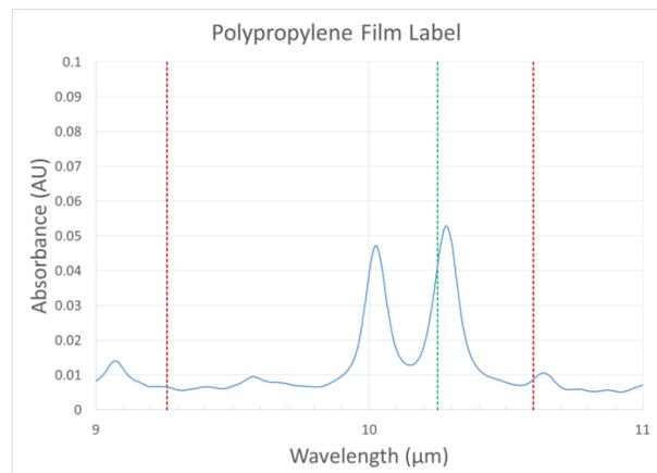
Figure 2: A measured FT-IR absorbance curve of a polypropylene label. From left to right, the 3 vertical lines
