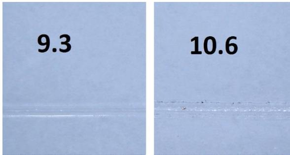
Figure 6: Clear cut edges are compared at 9.3 and 10.6  $\mu\text{m}$  wavelengths at 40X magnification. The 10.6  $\mu\text{m}$  cuts are rough and not as consistent.
