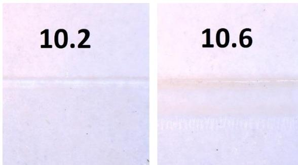
Figure 3: Clear PP cut edges are compared at 10.2 and 10.6  $\mu\text{m}$  wavelengths at 40X magnification. The yellow discoloration seen at 10.6  $\mu\text{m}$  was clearly visible even with the naked eye. The secondary line in the image on the right is vapour residue trapped between the label and liner.
