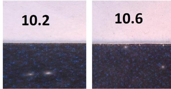
Figure 4: Opaque PP cut edges are compared at 10.2 and 10.6  $\mu\text{m}$  wavelengths at 40X magnification. Slight damage to the dark ink is seen in the image on the right.
