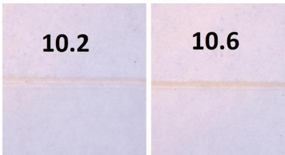
Figure 7: Paper with laminated PP cut edges are compared at 10.2 and 10.6  $\mu\text{m}$  wavelengths at 40X magnification
