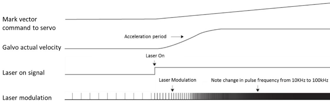
Fig. 2. Velocity Based Laser Modulation based on frequency. When the mark vector command (1<sup>st</sup> curve) starts and the laser is turned on (3<sup>rd</sup> curve), the galvo actual velocity (2<sup>nd</sup> curve) increases from zero and gradually reaches a constant value. The laser modulation signal (4<sup>th</sup> curve) is increased from 10kHz to 100kHz accordingly.
