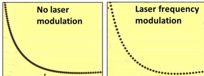
Fig. 3. Marking results of a corner with conventional control with no laser modulation (left) and with velocity-based laser modulation on frequency (right). Velocity-based laser modulation clearly improves the uniformity of laser density at the corner.
