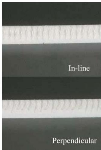
The pictures highlight the difference. Processing with the polarization perpendicular to the scribe direction causes a reduction in scribe depth and the tendency to produce the "hook" defect. Circular polarization offers mid ground - not as much penetration as parallel but consistency in all directions without showing the hook defect.
