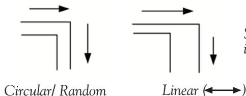
*Schematic of the effect of polarization, in terms of cut width and length of arrow indicating cut speed. Direction of linear polarization indicated in parenthesis.*
