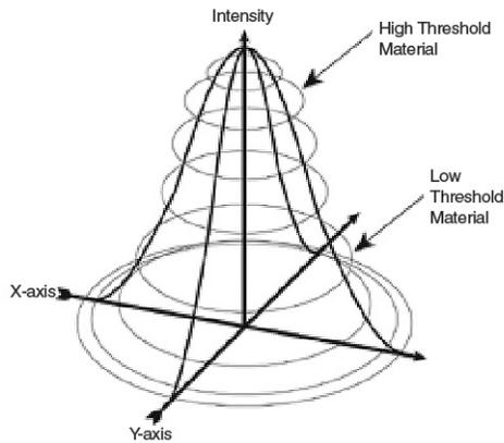
*As shown in this figure, the method of drilling a hole smaller than the spot size is to precisely control the laser's energy input in combination with a high threshold material.*
