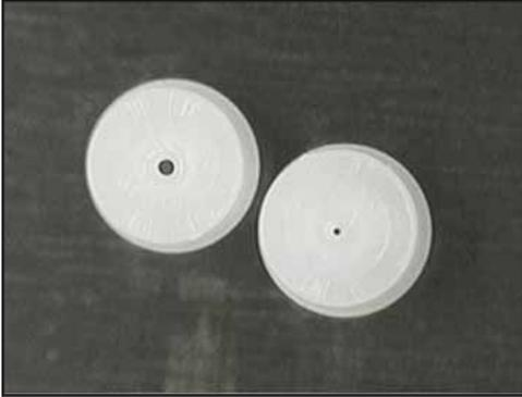
*In the case of the polyacetal plastic shown here, nozzle diameters ranged from 75 microns to over 300 microns. This variety of hole diameters is due to two features of the laser: (1) the gaussian mode of the beam, and (2) the fine energy input control.*
