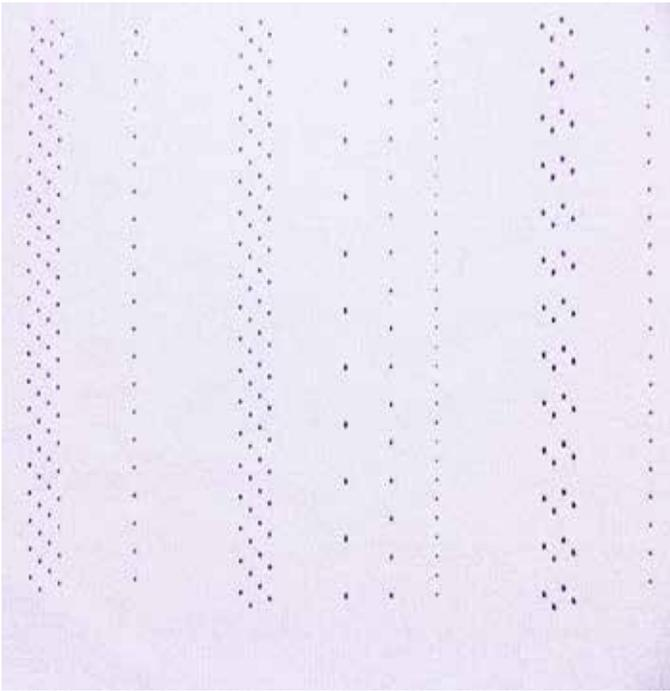
Figure 4: iPerforations at various frequencies in Polyester/Spandex
