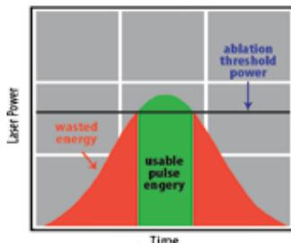
Long Pulse or Continuous Wave (CW) Laser
