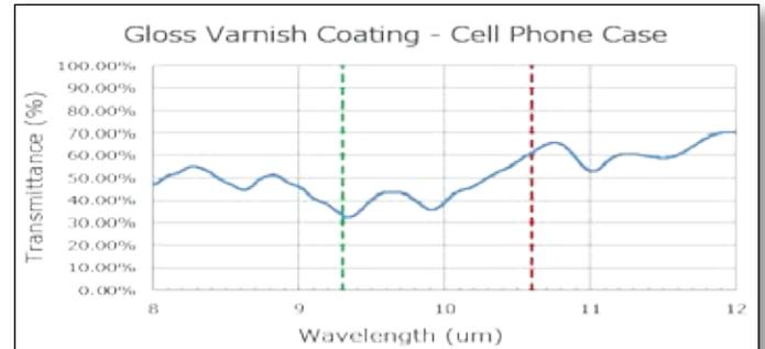
The transmission curve indicated that a laser at 9.3  $\mu\text{m}$  had 25% less transmission than the more common 10.6  $\mu\text{m}$  lasers available. The lower transmission rate would enable a Synrad laser to lightly mark the gloss coating at high speed while avoiding any damage to the underlying base plastic.
