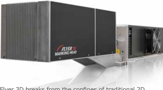
Flyer 3D breaks from the confines of traditional 2D marking head systems delivering an effective marking area roughly 2.5X the size of a 2 axis field with an equivalent spot size, up to 1084 mm x 993 mm. Flyer 3D uses a third servo-driven z-axis to dynamically focus the laser beam while maintaining a consistent spot size across the field. The result is sharp, detailed imagery or cutting over a larger area.
