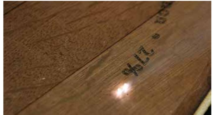
Marking large areas like this wine barrel lid is fast and easy with Flyer 3D. The servo-driven z-axis enables detailed imaging over a larger area. When combined with the right laser detailed imagery on target materials are achieved with no alignment needed between the laser and the marking head. Flyer 3D is a complete scanning head kit with fast, right-out-of-the-box set up, and easy operation.
