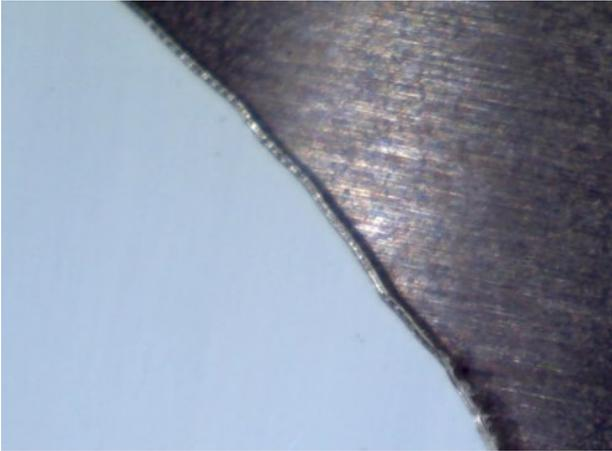
10.2  $\mu\text{m}$ : Cutting is 2.5X faster, and produces a crisp edge with minimal melt lip.
