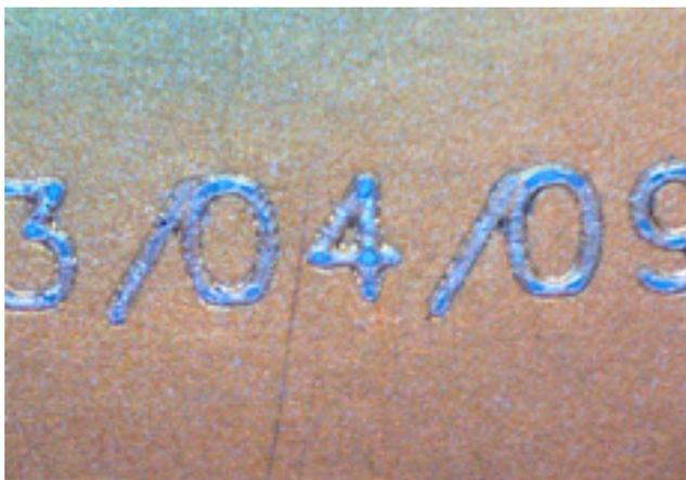
10.2  $\mu\text{m}$ : Clean, consistent, and highly visible mark.
