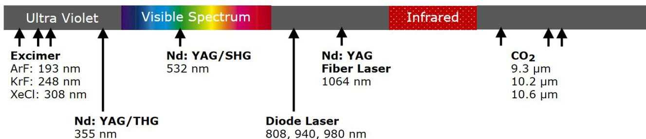
CO<sub>2</sub> lasers have long wavelengths, around 9.3 – 10.6 μm, with 10.6 μm as the most common. These wavelengths pair nicely with the absorption spectrum from polymers, ceramics, textiles, natural materials like paper or wood, and certain metals. By contrast, the shorter wavelength YAG or Fiber lasers tend to have better absorption in metals.
