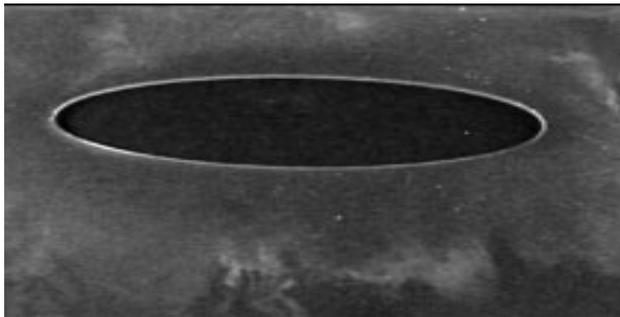
9.3  $\mu\text{m}$ : Cutting produces a clean edge with no residue and minimal melting.
