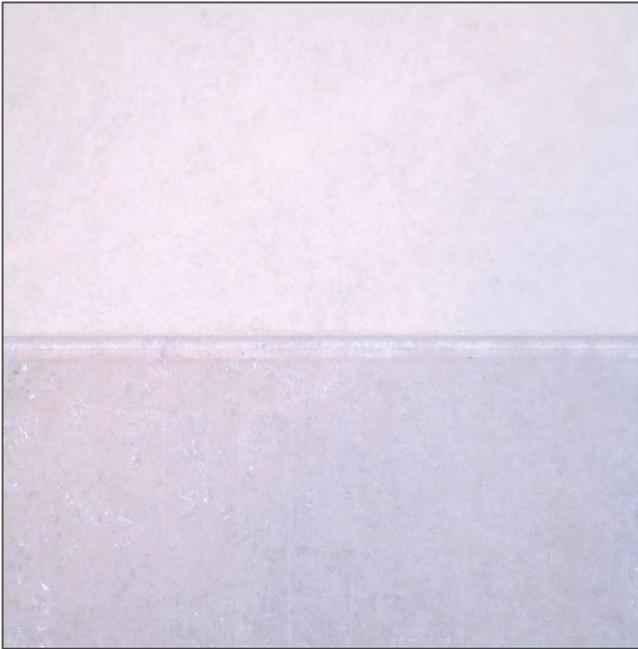
Clear label cut edge 10.2  $\mu\text{m}$  wavelength
